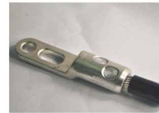
Fig.4 Smooth off any sharp edges
